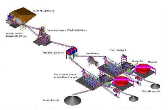
\*Please note that the above diagram shows the wash plant design including the second wash plant (Module 2) which has not been constructed as at the date of this Prospectus.
